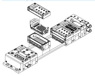
The mechanical connection between the CPX modules is established using tie rods. Two screws in the end plates are all that are needed to assemble the
