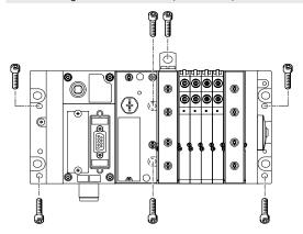
The MPA-L valve terminal is screwed onto the mounting surface using four M4 and two M6 screws or using six M6 screws. The mounting holes are on the left-hand and right-hand end plate and on the pneumatic interface.
