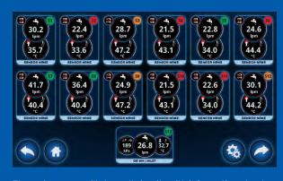
The main screen will show all circuits with information about flow and temperature. The main inlet and outlet will also show including pressure.
