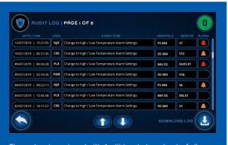
The system is equipped with Audit Log to keep track of all events including user ID tracer.
